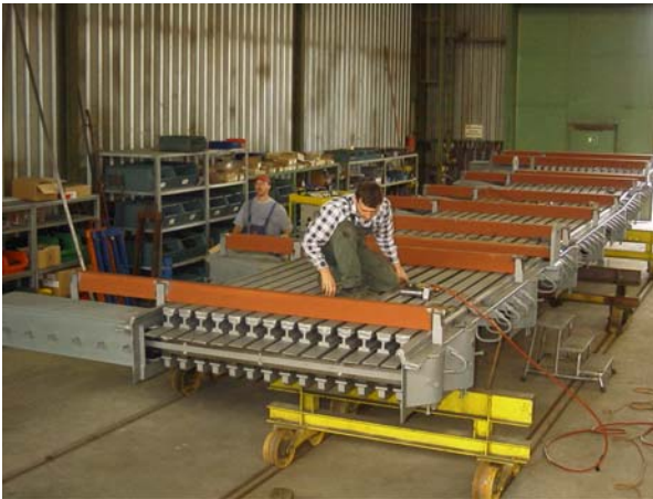
Fig. 1: Joint manufacture in the workshop
